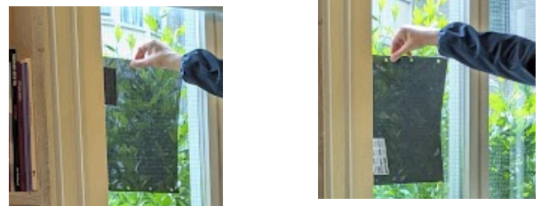
Figure 21: resp. 10% and 5% light transmittance shades
