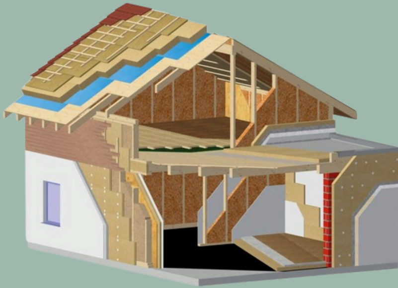
Figure 12: Possible insulation layer structures
